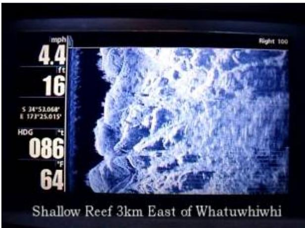
Fig. 7. Single-sided sidescan image of shallow high-relief rock.
